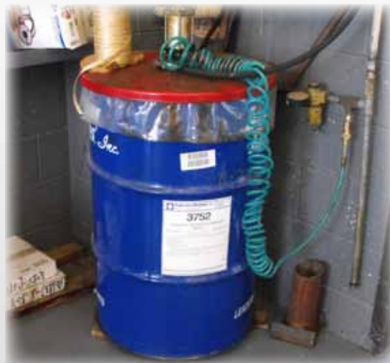
The shop uses Almagard Vari-Purpose Lubricant from an air-operated pump in a barrel.
