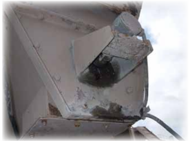
Spiral conveyor end shaft bearing using 3751.
